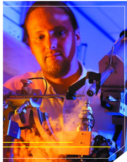
Conn Mallett aligns a CryoJet for an X-ray diffraction experiment.
